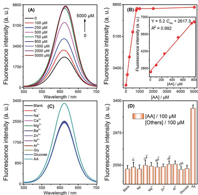
**Fig. 2** The analytical performance and selectivity of this sensor for AA detection. (A) and (B) Fluorescence spectra and calibration curve for AA detection. Inset: A linear relationship of the fluorescence signal versus the concentration of AA ranging from 0 to 800  $\mu\text{M}$ . (C) and (D) Fluorescence spectra and fluorescence signal of different interferents. All concentrations were 100  $\mu\text{M}$ . Error bars were estimated from at least three replicate measurements.
