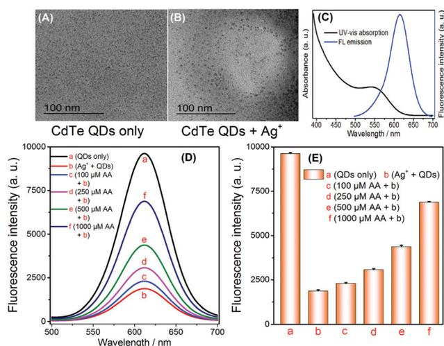
**Fig. 1** TEM images of CdTe QDs before (A) and after (B) the addition of  $\text{Ag}^+$  in the quenching reaction. (C) The spectra of the UV-vis absorption (black curve) and the fluorescence emission (FL, blue curve) of the CdTe QDs. (D) and (E) Both show the feasibility of the AA assay based on the controlled generation of Ag NPs and selective quenching reaction.
