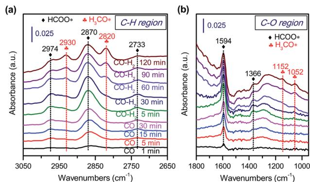
Fig. 12 *In situ* DRIFT spectra for the conversion of CO on Zn-ZrO<sub>2</sub> catalyst. (a) C-H region in 3050–2650 cm<sup>-1</sup>. (b) C-O region in 1800–1000 cm<sup>-1</sup>.
