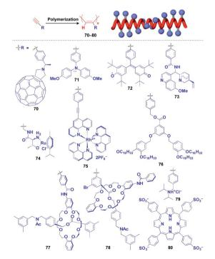
Fig. 12 Schematic structure of a polyacetylene-based helical 1D supramolecular scaffold (red) and examples of functional molecular units (blue) assembled with the scaffold.
