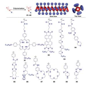
Fig. 13 Schematic structure of a polyisocyanide-based helical 1D supramolecular scaffold (red) and examples of functional molecular units (blue) assembled with the scaffold.
