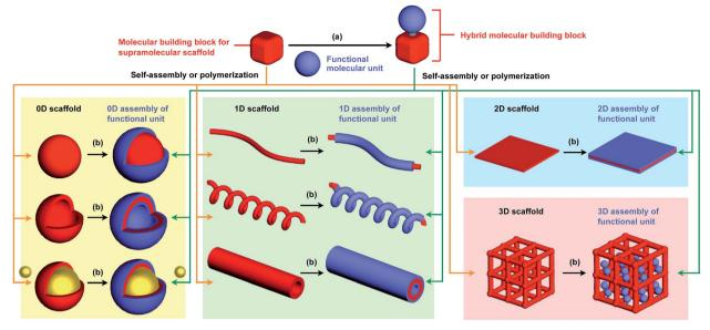
Fig. 1 Schematic illustration of the types of supramolecular scaffolds for the controlled assembly of functional molecular units into well-defined OD, 1D, 2D and 3D structures. (a) Pre-functionalization and (b) post-functionalization.
