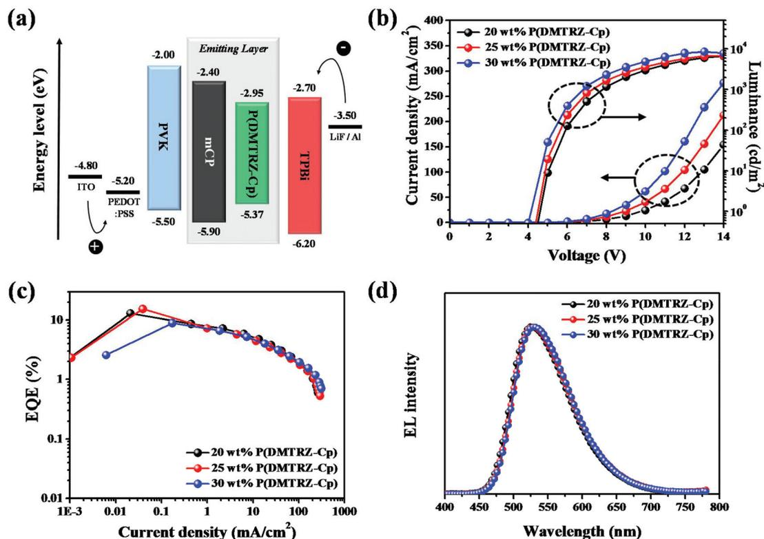
Fig. 4 (a) Schematic energy level diagram of a device with mCP as the host, (b) current density–voltage–luminance ( $J$ – $V$ – $L$ ) curves, (c) external quantum efficiency (EQE)–current density ( $\eta_{\text{ext}}$ – $J$ ) curves and (d) electroluminescence (EL) spectra at a luminance of  $1000 \text{ cd m}^{-2}$  of TADF-OLEDs fabricated using the new P(DMTRZ-Cp) polymer emitter.
