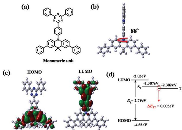
**Fig. 2** (a) Conjugated monomeric unit in P(DMTRZ-Cp). (b) Optimized geometry. (c) HOMO and LUMO spatial distributions and (d) energy level diagram for the conjugated unit in P(DMTRZ-Cp) calculated at the B3LYP/6-31G (DFT) level of theory with Gaussian 09W.
