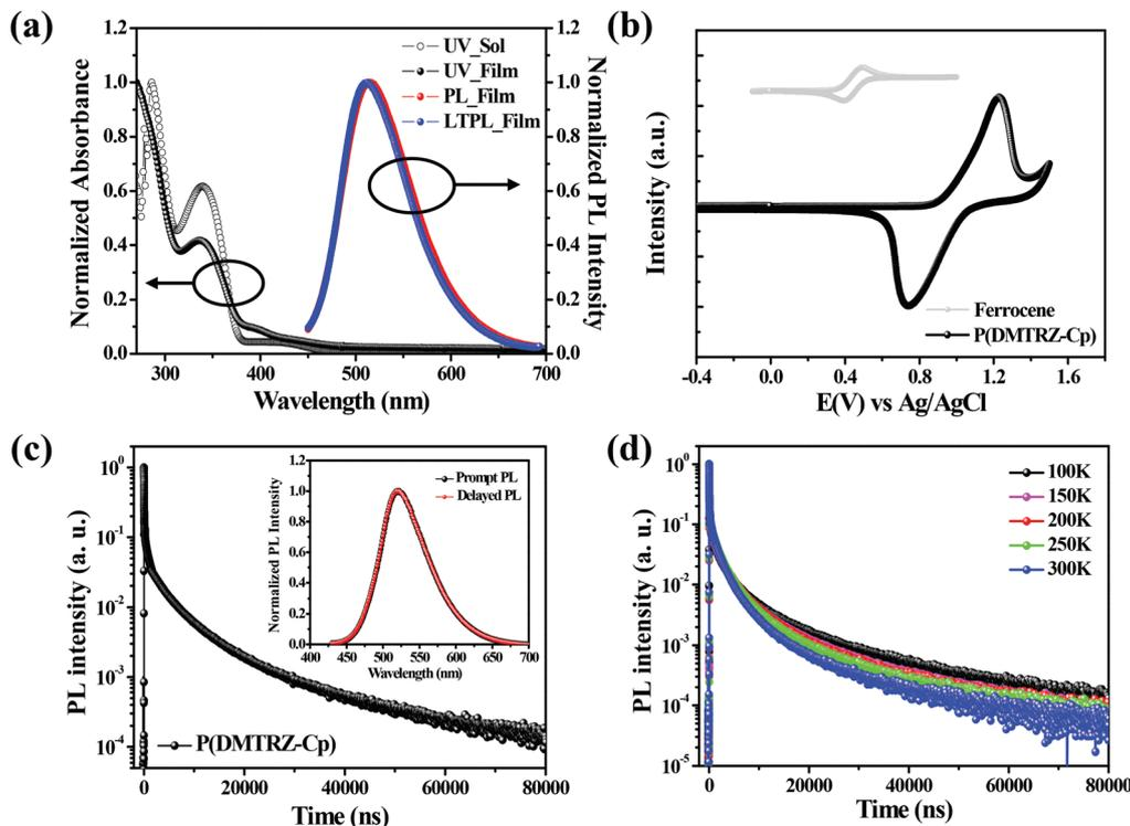
**Fig. 3** (a) UV-vis absorption spectra, photoluminescence (PL) and low-temperature PL (LTPL) spectra, (b) cyclic voltammogram of the P(DMTRZ-Cp) film. (c) Transient photoluminescence decay curve of the P(DMTRZ-Cp)-doped mCP film at 300 K; the inset is its prompt and delayed emission spectra. (d) Temperature-dependent transient PL decay curves over the 100 to 300 K temperature range for the P(DMTRZ-Cp)-doped mCP film.
