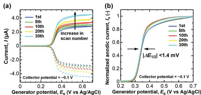
Fig. 8 (a)  $I_a$  (solid line) and  $I_c$  (dashed line) in 30 times repeated dual-mode CV of DA (100  $\mu\text{M}$ ) in PBS (pH 7.4) with the CNTF-IDE ( $W_e = 2 \mu\text{m}$  and  $W_g = 3 \mu\text{m}$ ) at  $\nu = 10 \text{ mV s}^{-1}$ . (b) Normalized  $I_a$  by that at 0.7 V.
