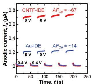
**Fig. 5** Anodic current ( $I_a$ ) at the generator in the dual-mode CA with the Au-IDE or the CNTF-IDE ( $W_e = 2 \mu\text{m}$  and  $W_g = 3 \mu\text{m}$ ). The generator potential was fixed at 0.4 V, and the collector potential was stepped as shown in the graph (0 V and 0.4 V). The potential is the value against the Ag/AgCl reference electrode.
