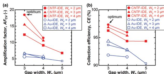
Fig. 4 (a) The amplification factor ( $AF_{CV}$ ) and (b) the collection efficiency (CE) with CV with different electrode structures. The data with the optimum electrode structure ( $W_e = 2$   $\mu\text{m}$  and  $W_g = 3$   $\mu\text{m}$ ) are shown with arrows.
