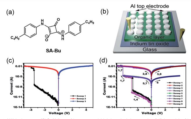
Fig. 1 (a) Molecular structure of SA-Bu, (b) diagram of the prototype sandwich device, and typical current-voltage (I-V) characteristics of the (c) binary and (d) ternary devices
