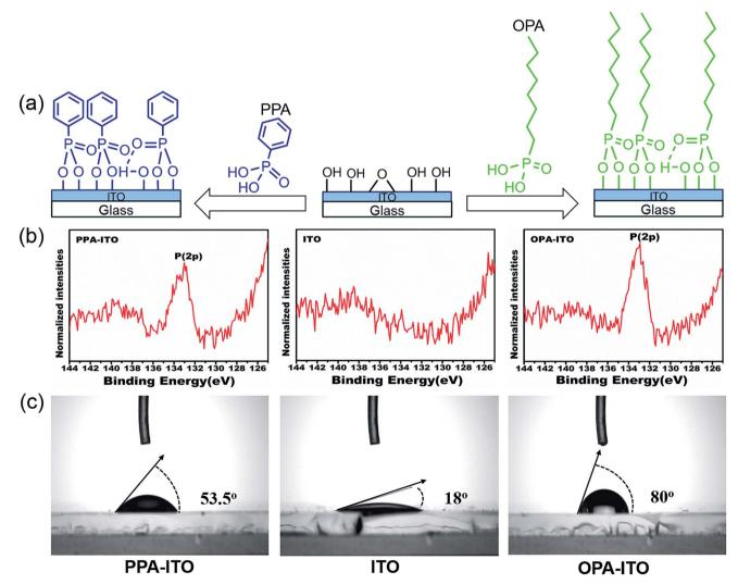
Fig. 2 (a) Process of surface modification by phosphonic acids on the surface of ITO glass; (b) XPS spectra of P(2p) of PA-modified ITO substrates; (c) wettability tested in air.
