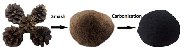
Fig. 1 Schematic diagram of synthesis route of PHC sample.
