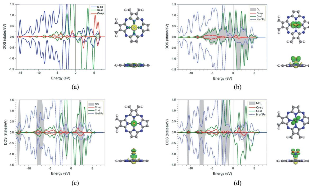
**Fig. 2** DOS (left panel) and electron density difference in top- and side-views (right panel) of (a) CrPc (b) O<sub>2</sub> adsorbed CrPc, (c) NO adsorbed CrPc and (d) NO<sub>2</sub> adsorbed CrPc. The green and yellow regions represent electron density accumulation and depletion regions, respectively. The isosurface value is  $\pm 0.02$ .
