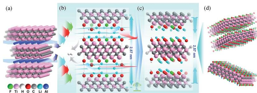
Fig. 4 Schematic diagram of the structural formation mechanism for the  $\text{Ti}_3\text{C}_2\text{T}_x$  sample. The atomic structure was built along the [110] direction. Atomic arrangements of (a) the  $\text{Ti}_3\text{AlC}_2$  structure, (b) the as-synthesized  $\text{Ti}_3\text{C}_2\text{T}_x\text{-Li}$  sheets, (c) storing in air for 50 days, and (d) one and two layers structures.
