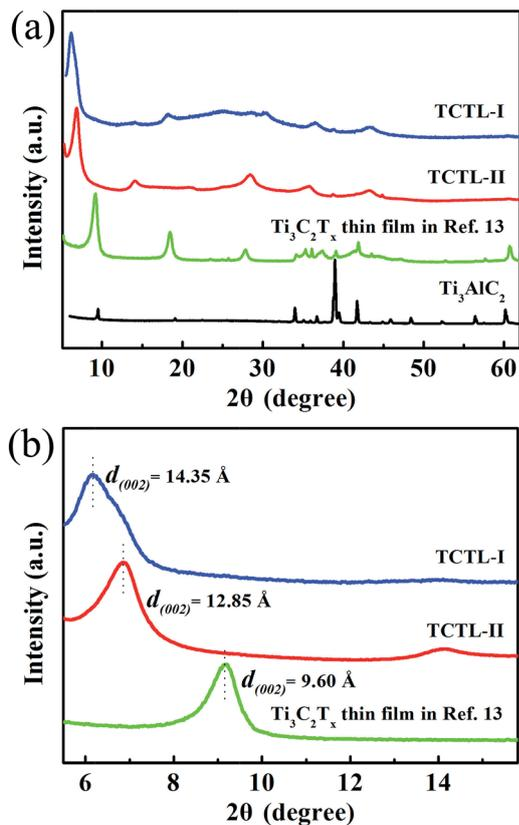
Fig. 2 (a) XRD patterns of the TCTL-I, TCTL-II, the previous  $\text{Ti}_3\text{C}_2\text{T}_x$  thin film in ref. 13, and  $\text{Ti}_3\text{AlC}_2$  powder and (b) the corresponding enlarged XRD patterns.
