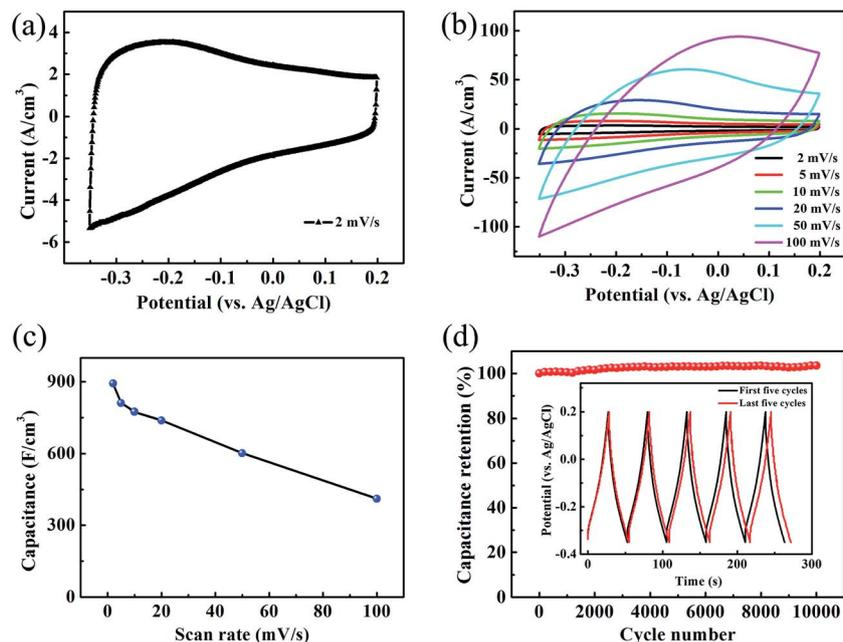
Fig. 5 The results of TCTL-II (a) at a scan rate of  $2 \text{ mV s}^{-1}$ , and (b) at different scan rates. (c) Volumetric capacitance as a function of scan rate. (d) The cycling performance of the TCTL-II electrode at a current density of  $5 \text{ A g}^{-1}$ . The black and red GCD voltage profiles of the TCTL-II electrode shown in the inset represent the first five cycles and the last five cycles, respectively.
