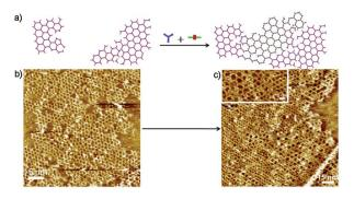
Fig. 6 (a) A schematic diagram of the formation of 2DP heterostructure on the surface. STM images of the submonolayer of  $2DP_{1+3}$  (b) and *in situ* synthesized hetero-structure of  $2DP_{1+3}/2D_{1+4}$  (c) at the octanoic acid/HOPG interface. Imaging conditions: (b)  $I_{\rm set}=28$  pA,  $V_{\rm bias}=0.68$  V; (c) and inset  $I_{\rm set}=27$  pA,  $V_{\rm bias}=0.52$  V.
