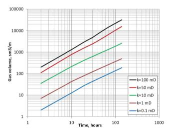
Fig. 16 Temporal profile of cumulative gas volume generated per  $1\,\mathrm{m}$  thickness of MH layer with various permeability values.
