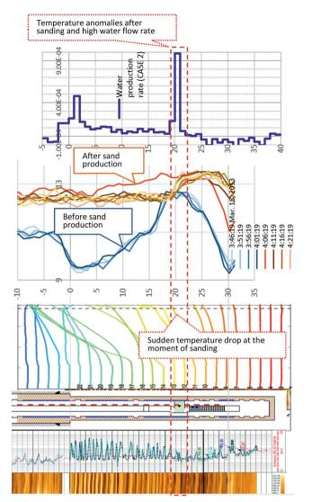
Fig. 17 Comparison of temperature data from monitoring and production boreholes and the water flux evaluated by the optimization processes. The depth of the significant temperature change in the monitoring boreholes (18–20 mBTMHCZ, the boundary of Units IV-1 and IV-2) corresponds to the zone of temperature discontinuity in the production hole and the zone of strong water flow.
