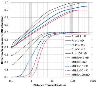
Fig. 15 Radial profiles of dimensionless pressure P and MH saturation change  $\Delta S_{\rm h}$  for different lithologies and permeability values ( $k=0.1-100~{\rm mD}$ ) at the elapsed time  $t=140~{\rm hours}$  computed with ondimensional axisymmetric non-isothermal model. The initial hydrate saturation  $S_{\rm h0}$  is set to be 0.6. The result illustrated is from the non-isothermal model.
