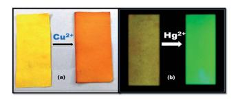
Fig. 11 (a) Naked eye detection on a piece of paper soaked with FDNS: from left to right FDNS (blank); FDNS + Cu<sup>2+</sup> (b) the variation of the color of FDNS coated on filter paper before (left) and after treatment with Hg<sup>2+</sup> (right) under UV excitation light.
