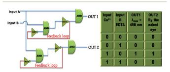
Fig. 9 Truth table and sequential logic circuits displaying memory units with two inputs (input A (Cu<sup>2+</sup>) and input B (EDTA)) and two outputs in the presence of chemical inputs.
