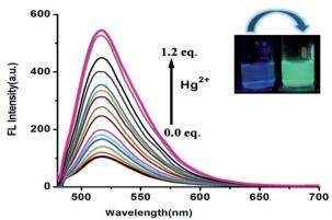
Fig. 5 Fluorescence spectral titrations of FDNS (10  $\mu$ M) in aqueous : MeOH (8 : 2 v/v) HEPES buffer (1 mM, pH 7.4) on the incremental addition of Hg(NO<sub>3</sub>)<sub>2</sub> (1.2 equiv.)  $\lambda_{\rm ex}=465$  nm. Inset: the colour change of FDNS solution in the presence of Hg<sup>2+</sup> ions under UV light.
