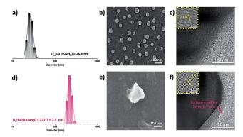
Fig. 2 DLS diagrams, FE-SEM, and FE-TEM images of GQD-NH<sub>2</sub> (a-c) and GQD-comp (d-f). Pre-dried samples were dispersed in DW at  $0.1 \,\mathrm{mg}\,\mathrm{mL}^{-1}$  (for DLS and TEM) and  $0.25 \,\mathrm{mg}\,\mathrm{mL}^{-1}$  (for SEM). The insets show low-magnification (top) and FFT filtered TEM images (bottom).
