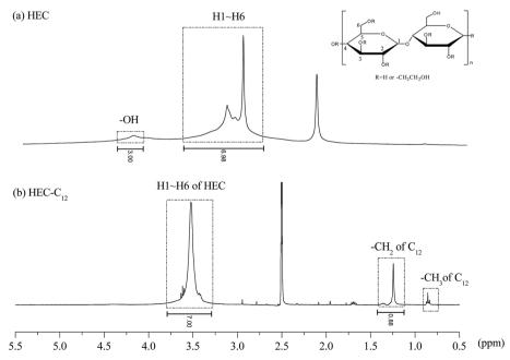
Fig. 1  $^{1}$ H NMR spectra of HEC (a) and HEC-C<sub>12</sub> (b) recorded at 400 MHz in DMSO-d<sub>6</sub> at room temperature
