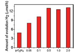
Fig. 20 Photocatalytic activity of F-doped  $g-C_3N_4$  towards HER from water/TEA under visible light ( $\lambda > 420$ ) (reproduced from ref. 47, licence number 3767471256893).
