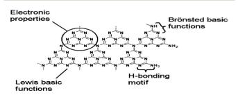
Fig. 2 Structure of planar  $q-C_3N_4$  (reproduced from ref. 11).
