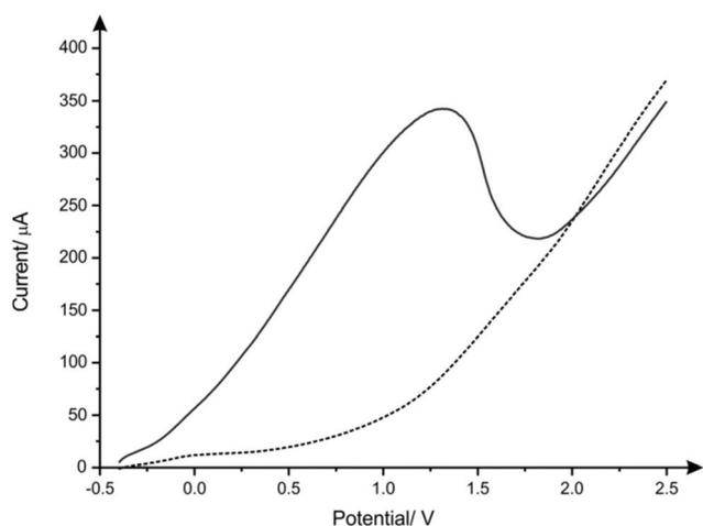
**Fig. 1** Linear sweep voltammograms using CuSPEs in the absence (dashed line) and presence of 1 mM sulfide (solid line) in pH 8 B–R buffer solution. Deposition time and potential of 60 s at  $-0.4$  V respectively (vs. Ag/AgCl) and scan rate  $100 \text{ mV s}^{-1}$ .
