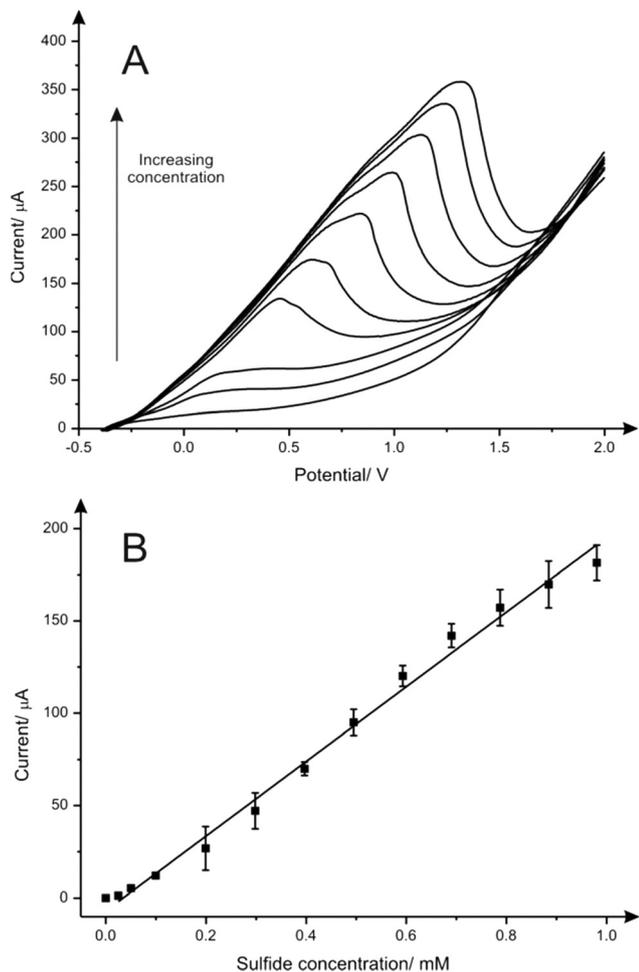
**Fig. 2** (A) LSV of a CuSPE towards increasing concentration of sulfide over a range of 0.0 to 0.1 mM at pH 7 PBS. Deposition time and potential of 60 s at  $-0.4$  V respectively (vs. Ag/AgCl), scan rate  $100$   $\text{mV s}^{-1}$  applied between each addition. (B) The corresponding calibration plot ( $N = 3$ ).
