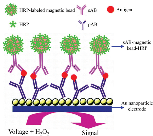
Fig. 8 AuNP based electrochemical immunosensor (adapted with permission from ACS Nano , 2009, 3, 585–594. Copyright (2009) American Chemical Society).
