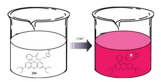
Fig. 260 Chemical structure of probe 296, proposed ligand–Hg<sup>2+</sup> binding mechanism and bioimaging applications.
