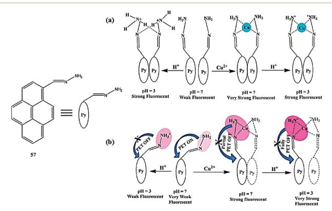
Fig. 49 Chemical structure of receptor 57 and the proposed mechanism for the effect of pH variation on the excimer (a) and monomer (b) emission of 57 in the absence and presence of Cu<sup>2+</sup> ions.
