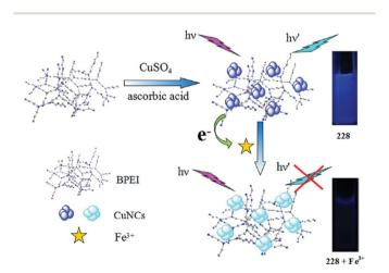
Fig. 192 Synthetic strategy of the BPEI–CuNCs and the mechanism of the BPEI–CuNCs probe for  ${\rm Fe^{3+}}$  sensing.
