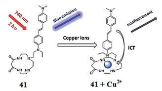
Fig. 37 Chemical structure of probe 41 and the proposed copper complexation mechanism.
