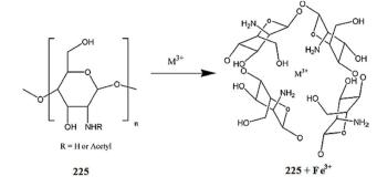
Fig. 189 Schematic of the Fe-chitosan complex formation.
