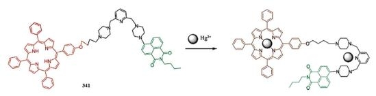
Fig. 301 Chemical structure of ligand 341 and the proposed ligand binding mechanism.
