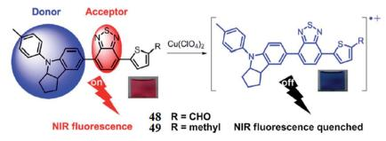
Fig. 44 Chemical structure of sensor 48 and 49 and copper-induced radicalization.
