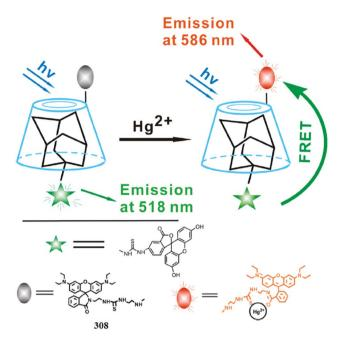
Fig. 270 Schematic for the formation of the FRET-based ratiometric sensing system for  $Hg^{2+}$  with  $\beta$ -CD as the vehicle.
