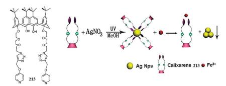
Fig. 178 Chemical structure of calix[4] arene 213, synthesis of 213-Aq NPs and schematic of Fe<sup>3+</sup>-induced 213-Aq NP aggregation.
