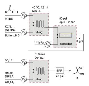
Scheme 2 Schematic representation of the flow setup.
