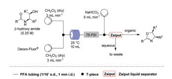
Scheme 1 Ontimised conditions for the flow synthesis of oxazolines
