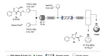
Scheme 3 Platform set up for the scale up experiment.
