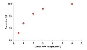
Fig. 2 Effect of flow rate on cyclodehydration of 1a to 2a (residence time = 1.7 min
