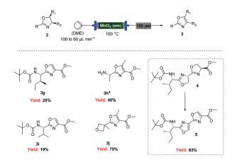
Scheme 5 Flow oxidation of 2-alkyl-oxazolines using amorphous MnO<sub>2</sub>. a Deprotection was observed.
