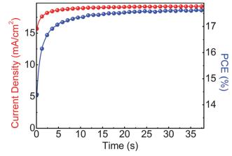
Fig. 3 Stabilized current density and power output measured close to the maximum power point ( $\sim$  0.92 V) for a photovoltaic device of glass/FTO/TiO $_X$ /60-PCBM/CH $_3$ NH $_3$ Pbl $_3$ /spiro-MeOTAD/Au.
