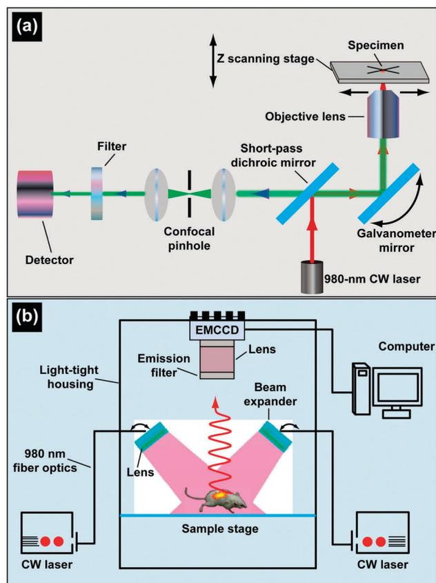
Fig. 22 Schematic setup used for *in vitro* and *in vivo* imaging of cells and animals. (a) Schematic illustration of a laser scanning UC luminescence confocal microscope for *in vitro* study. (b) Experimental setup for *in vivo* imaging of small animals using UC nanocrystals as biomarkers. (Reprinted with permission from ref. 173 and 246. Copyright 2009, American Chemical Society.)
