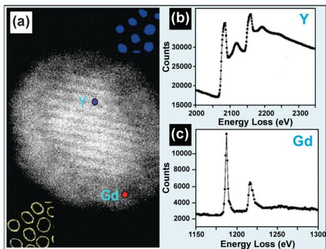
Fig. 12 EELS technique for composition characterization of UC nanocrystals. (a) HADDF image of a single NaYF<sub>4</sub>:Yb/Er (20/2 mol%)@NaGdF<sub>4</sub> core-shell nanocrystal. (b and c) EELS spectra of yttrium L<sub>2,3</sub> and gadolinium M<sub>4,5</sub> edges obtained from the NaYF<sub>4</sub>:Yb/Er (20/2 mol%) core and NaGdF<sub>4</sub> shell as labeled in a. (Reprinted with permission from ref. 134. Copyright 2012, American Chemical Society.)
