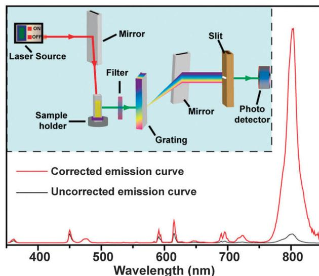
Fig. 17 Emission spectrum of NaGdF<sub>4</sub>:Yb/Tm (49/1 mol%)/NaGdF<sub>4</sub>:Eu (15 mol%) nanocrystal colloidal solution (in cyclohexane) measured by a red-sensitive photomultiplier before and after detector correction. The inserted shows a schematic layout of the luminescence spectrophotometer.
