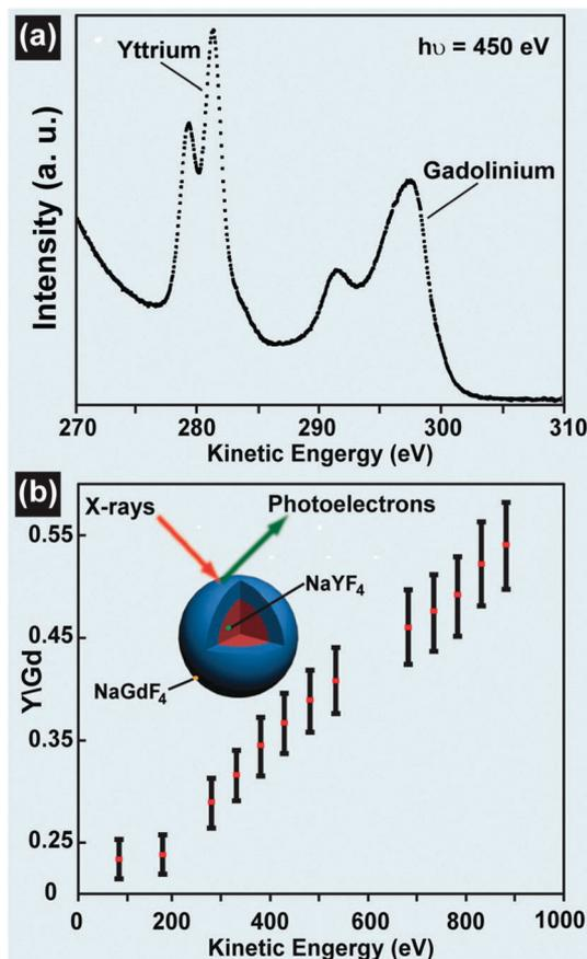
Fig. 13 Composition characterization of UC nanocrystals by XPS technique. (a) Signals of yttrium 3d and gadolinium 4d core levels from NaGdF<sub>4</sub>@NaYF<sub>4</sub> nanocrystals before the subtraction of the background ( $h\nu = \text{ca. } 450$  eV). (b) Intensity ratio of yttrium (3d) to gadolinium (4d) core levels as a function of photoelectron kinetic energy. (Reprinted with permission from ref. 168. Copyright 2009, American Chemical Society.)
