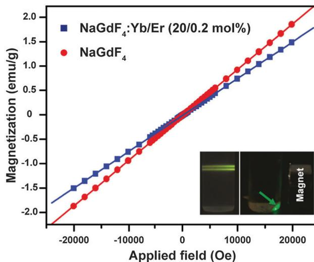
Fig. 24 Magnetization of NaGdF<sub>4</sub>:Yb/Er (20/0.2 mol%) and NaGdF<sub>4</sub> nanocrystals as a function of the applied field. Note that inset shows luminescent photographs of NaGdF<sub>4</sub>:Yb/Er nanocrystals, recorded under excitation at 980 nm, with and without a magnet, indicating that these UC nanocrystals can be recovered by applying an external magnetic force. (Reprinted with permission from ref. 256. Copyright 2011, American Chemical Society.)
