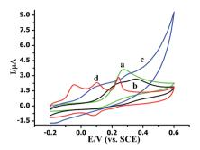
Fig. 2 Cyclic voltammograms of (a) bare GCE and (b) AuNPs/GCE (c) MoS $_2$ /GCE (d) AuNPs@MoS $_2$ /GCE in 0.1 M PB solution (pH 7.0) containing of 20 mM AA, 1  $\mu$ M DA and 10 mM UA. Scan rate: 100 mV s $^{-1}$ .
