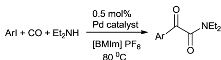
Scheme 70 Reagents and conditions: microflow system: aryl iodide (14.0 mmol), Et 2 NH (70 mmol, 5.0 equiv.), CO (20 or 15 atm), Pd cat. (0.5 mol%) in [BMIm]PF 6 (17 mL); flow rates: mixture of aryl iodide and Et 2 NH (0.04 mL min -1 ), Pd/[BMIm]PF 6 (0.14 mL min -1 ), CO (0.25 mL min -1 ), temp. 80 °C, residence time 34 min; conventional batch system: aryl iodide (2.66 mmol), Et 2 NH (5.0 equiv.), Pd cat. (0.5 mol%), [BMIm]PF 6 (2.0 mL), CO (20 or 15 atm), 80 °C, time 5 h.
