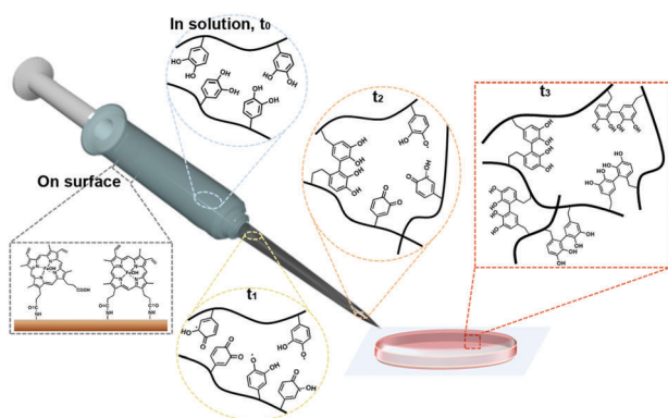
Scheme 1 Schematic diagram of the preparation of catalyst-free injectable hydrogels produced by the interfacial chemical activation of surface-immobilized hematin. Via an interfacial reaction between the catechol-containing polymers ( t_0 ) and the immobilized hematin in the syringe (shown in gray), the tethered catechol moieties become active intermediates ( t_1 – t_2 ). Finally, the intermediates react with each other, forming catalyst-free hydrogels ( t_3 ).
