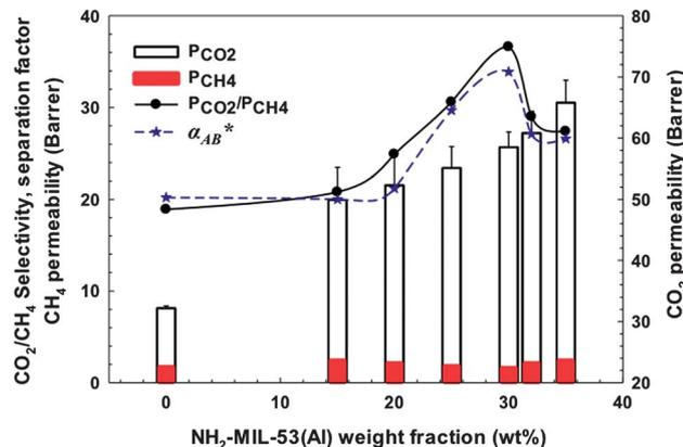
**Fig. 11** CO<sub>2</sub> and CH<sub>4</sub> permeabilities, ideal selectivity ( $P_{\text{CO}_2}/P_{\text{CH}_4}$ ) and separation factor ( $\alpha^*$ ) for CO<sub>2</sub> : CH<sub>4</sub> = 50 : 50 as a function of NH<sub>2</sub>-MIL-53(Al) loading at 308K and 150 psi for 6FOD(11) + 2%-MOF MMMs.
