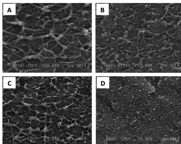
**Fig. 5** SEM micrographs of 6FOD(11) + 2% with (A) 20 wt%; (B) 25 wt%; (C) 30 wt%; and (D) 35 wt% of NH<sub>2</sub>-MIL-53(Al).
