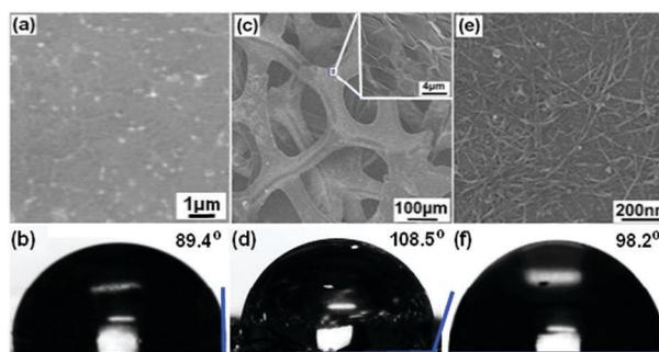
**Fig. 1** SEM images, and optical images of a water droplet placed onto the surface, of a 2D graphene film (a, b), 3D graphene foam (c, d) and a 2D CNT network film (e, f). The inset of (c) shows the SEM image of the graphene skeleton surface.
