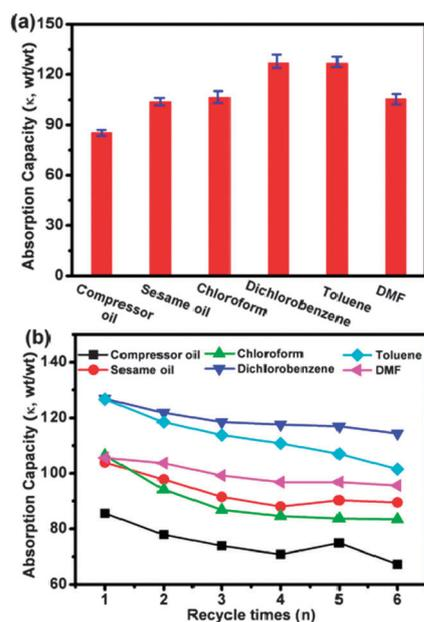
**Fig. 5** (a) Oil and organic solvent absorption capacities of the graphene–CNT hybrid foams. The error bars indicate the standard deviations from 3 samples. (b) Absorption recyclability of the graphene–CNT hybrid foams for oils and organic solvents.
