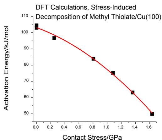
Fig. 3: Plot of the activation energy calculated by DFT as a function of contact stress for the normal-stress-induced mechanochemical decomposition of methyl thiolate species adsorbed on Cu(100).
