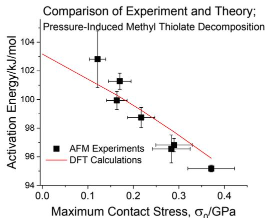
Fig. 4: The experimental data are shown plotted directly as reaction activation energy versus maximum contact stress, compared with the results of DFT calculations (—).
