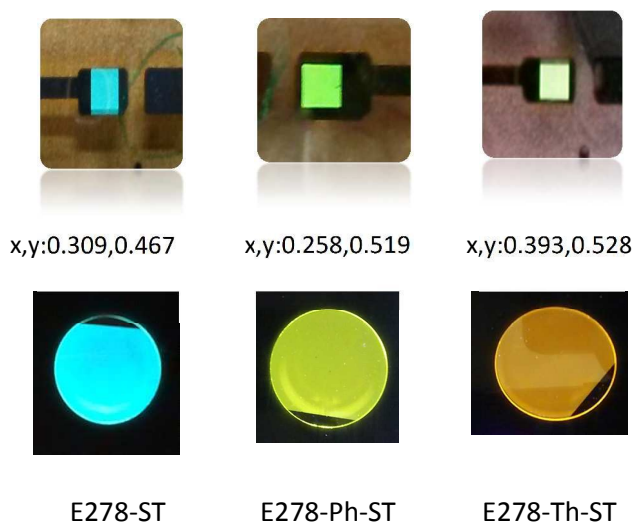
Figure 11 Single layer electroluminescent devices of E278-ST, E278-Ph-ST, E278-Th-ST (top), CIE x,y colour coordinates and the photoluminescence of thin films under 365 nm irradiation (bottom)
