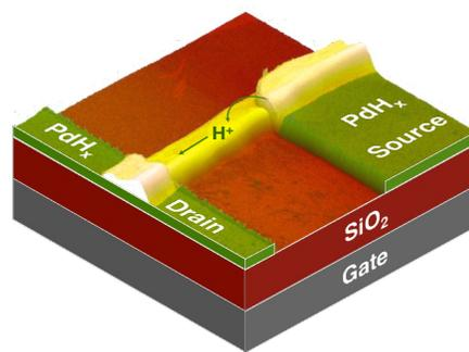
**Figure 1.** Schematic of a protonic device, in this case a protonic field effect transistor ( $H^+$ -FET). A  $PdH_x$  source and drain inject and drain  $H^+$  into and from a biopolymer or organic polymer. A potential applied to a back gate, which is insulated from the polymer with a  $SiO_2$  layer modulates the source drain current in transistors. AFM image of maleic chitosan thin film (false coloured) overlaid onto a back-gated FET structure. Reproduced from ref. 31.
