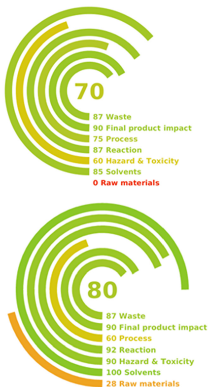
Fig. 5 Green Motion™ radar plots comparing the environmental profile of the traditional Claisen–Schmidt condensation (upper panel) and the developed MW-assisted solvent-free protocol (lower panel).
