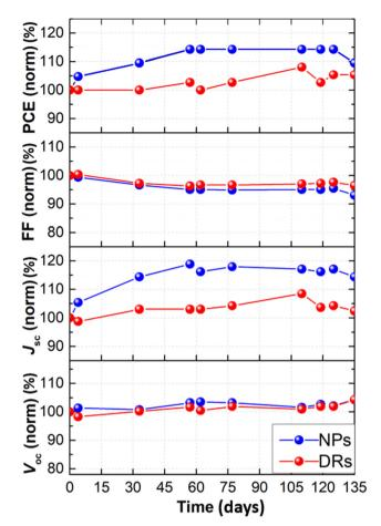
Fig. 6 Normalized photovoltaic parameters *versus* time for aqueous DSSCs prepared with DRs- and NPs-based photoanodes, stored under dark conditions and ambient temperature.
