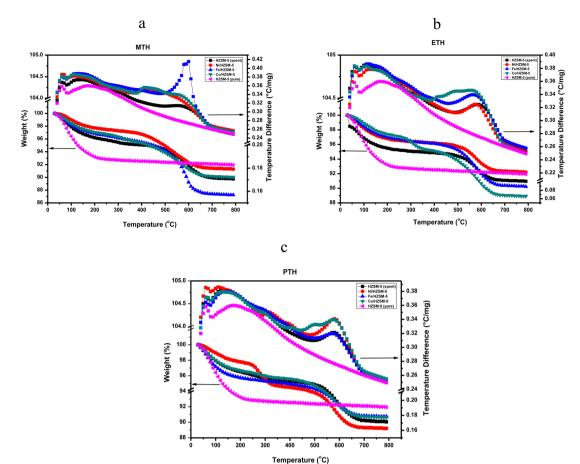
Fig. 6 TGA-DTA profile of (a) MTH, (b) ETH and (c) PTH conversion at T = 350 °C and WHSV = 7 h<sup>-1</sup>.
