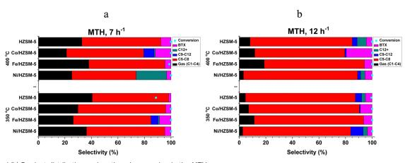
Fig. 1 (a) and (b) Product distribution and methanol conversion in the MTH process.
