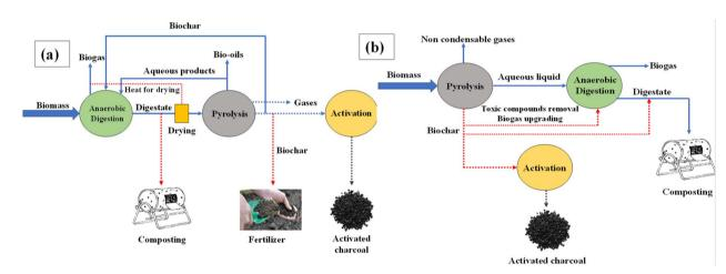
Fig. 4 (a) Flow diagram for hybrid AD and pyrolysis digestion process; (b) flow diagram for hybrid pyrolysis and AD digestion process.
