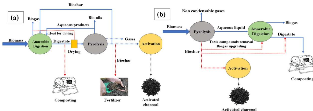
Fig. 4 (a) Flow diagram for hybrid AD and pyrolysis digestion process; (b) flow diagram for hybrid pyrolysis and AD digestion process.
