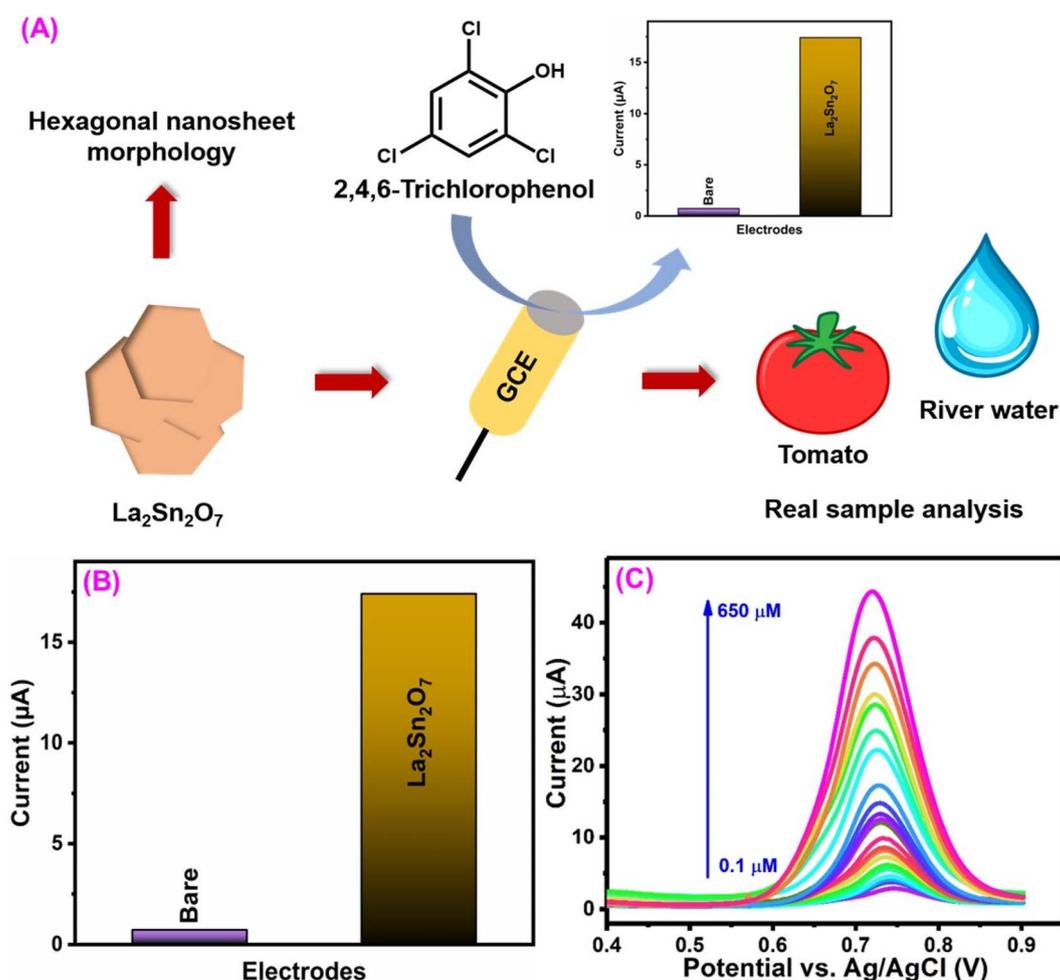
Fig. 8 (A) Schematic diagram for the synthesis of the  $\text{La}_2\text{Sn}_2\text{O}_7$  nanosheet and its electrochemical detection studies. (B) CV current response of the bare GCE and  $\text{La}_2\text{Sn}_2\text{O}_7$ /GCE towards TCL detection. (C) DPV response of  $\text{La}_2\text{Sn}_2\text{O}_7$ /GCE for detection of various concentrations of TCL<sup>124</sup> (modified). ((C) License number: 5570091012633).
