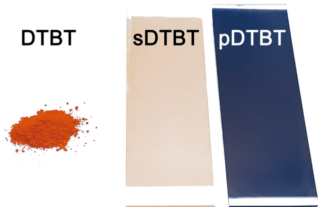
Fig. 1 Optical images of the DTBT monomer powder (orange), the sublimed sDTBT (0) coating (orange) and oCVD pDTBT (13) coating (blue) prepared from DTBT on glass substrates.
