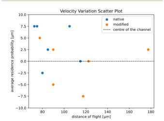
Fig. 5 Scatter plot of showing the RBC residence probability<sup>20</sup> of the RBC (distance from the channel centre line) against the distance of flight (which is proportional to the cell velocity). In the plot we used all RBCs shown in Fig. 3. The channel width at its widest section is 20  $\mu m$ .
