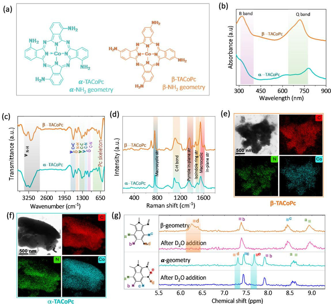
**Fig. 1** Molecular structures of isomeric (a)  $\alpha$ -TACoPc and  $\beta$ -TACoPc molecules. (b) UV-vis spectra. (c) ATR-FTIR spectra, and (d) Raman spectra of isomeric  $\alpha$ -TACoPc and  $\beta$ -TACoPc molecules. HRTEM images and elemental mapping of (e)  $\beta$ -TACoPc and (f)  $\alpha$ -TACoPc molecules. (g)  $^1\text{H}$  NMR spectra in  $\text{DMSO}-d_6$  for the isomeric molecules before and after  $\text{D}_2\text{O}$  addition.
