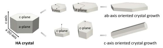
Fig. 4 Typical hexagonal HA crystal structure with the possible orientation growth on a, b or c planes.
