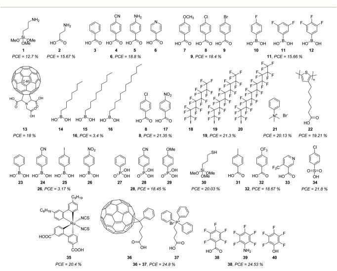
Commercial molecules are used for the formation of SAMs in PSCs, indicating the highest PCE obtained in each case.
