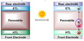
Fig. 1 Common architectures of PSCs (regular and inverted) and their working mechanism. h: holes, e: electrons.
