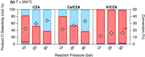
Fig. 4  $CO_2$  conversion (markers) and product selectivity (bars) of CZA, Ca/CZA, and K/CZA in the co-fed  $CO_2$  hydrogenation reaction at (a) T=150-250 °C at 30 bar and (b) P=10-30 bar at 250 °C. Reaction conditions: WHSV of 0.5  $g_{CO_2}$   $g_{cat}^{-1}$  h<sup>-1</sup> and H<sub>2</sub>:  $CO_2$  molar ratio of 3:1. Materials were pre-reduced in 95% H<sub>2</sub>/Ar for 16 h at 250 °C.
