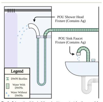
Fig. 1 Schematic of the building plumbing context for the use of Ag-POU devices, highlighting the source of biofilm in the drinking water system and intended function of silver in the POU device at the faucet or shower.
