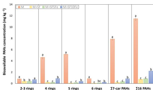
**Fig. 6** Bioavailable PAH concentrations of 2/3-ringed (2–3 rings), 4-ringed (4 rings), 5-ringed (5 rings), and 6-ringed (6 rings) in the untreated and treated M soil. Bars with the same letter do not differ significantly ( $p < 0.05$ ) within each PAH group.
