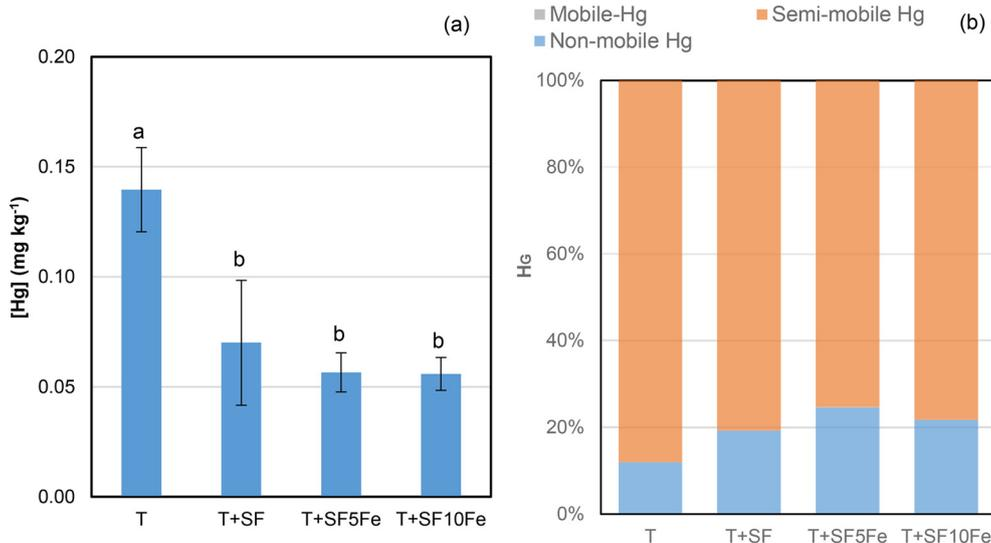
**Fig. 3** (a) Concentration of Hg in TCLP extracts and (b) fractionation of Hg following the USEPA Method 3200: mobile Hg, semi-mobile Hg and non-mobile Hg in the untreated and treated T soil. Bars with the same letter do not differ significantly ( $p < 0.05$ ).
