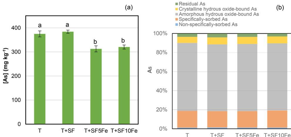
Fig. 2 (a) Concentration of As in TCLP extracts and (b) fractionation of As following an adopted sequential extraction method proposed by Wenzel *et al.*<sup>40</sup> non-specifically sorbed As, specifically sorbed As, amorphous hydroxide-bound As, crystalline hydroxide-bound As and residual As in the untreated and treated T soil. Bars with the same letter do not differ significantly ( $p < 0.05$ ).
