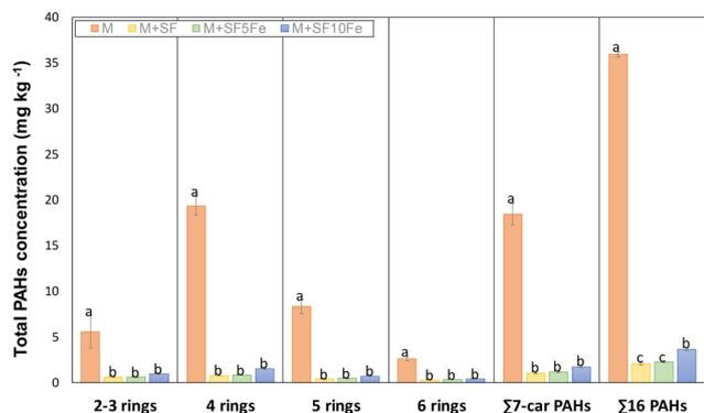
**Fig. 5** Total PAH concentration of 2/3-ringed (2–3 rings), 4-ringed (4 rings), 5-ringed (5 rings), and 6-ringed (6 rings) in the untreated and treated M soil. Bars with the same letter do not differ significantly ( $p < 0.05$ ) within each PAH group.
