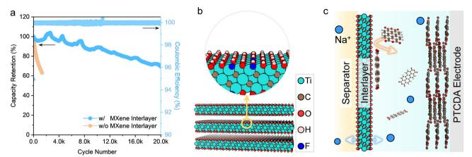
Fig. 5 Cycling stability tests. Cycling stability of the PTCDA electrode in the hybrid electrolyte ( $n_{NaClO_4}$ :  $n_{acetamide}$ :  $n_{water}$  = 1:4:4) with and without the MXene interlayer (current rate: 100C). Schemes of the 2D MXene nanosheets with negatively charged surfaces (b) and a cell configuration with the MXene interlayer to mitigate the dissolution of PTCDA during operation (c).
