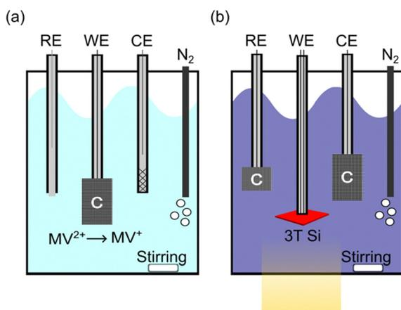
**Fig. 3** Schematic of the experimental set up for (a) the *in situ* pre-electrolysis of  $MV^{2+}$  to  $MV^+$  and (b) for photoelectrochemical/electrochemical characterization of 3T Si with respect to the  $MV^{2+}/MV^+$  solution potential using carbon cloth electrode (C).
