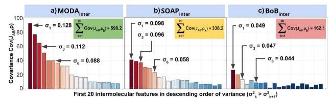
Fig. 7 Variance—covariance plots for intermolecular components of (a) MODA, (b) SOAP and (c) BoB with  $J_{AB}$ . The x-axis on each plot (and the color of each bar) corresponds to the variance of the 20 intermolecular features with highest variance, while the y-axis corresponds to the covariance of the component with  $J_{AB}$ . Insets show the cumulative covariance of all the plotted features.
