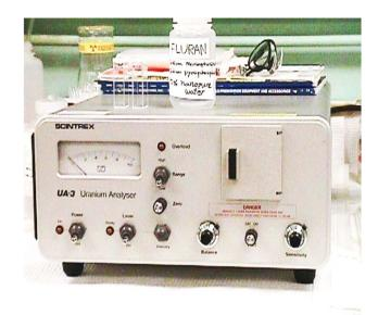
Fig. 1 UA-3 uranium analyzer (SCINTREX, Canada).
