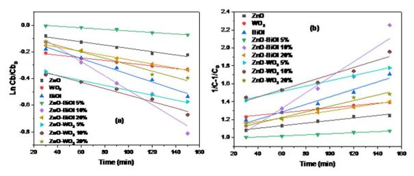
Fig. 7 (a) Pseudo-first-order kinetic model fit for 2-CBP degradation. (b) Pseudo-second-order kinetic model fit for 2-CBP degradation.
