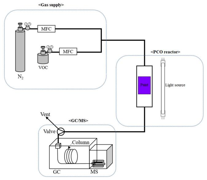
Fig. 1 Schematic diagram of the photocatalytic oxidation setup
