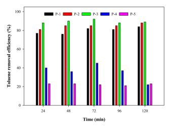
Fig. 3 The photocatalytic activity of paints P-1, P-2, P-3, P-4, and P-5 against 3 ppm toluene with a total flow rate of 50 mL min<sup>-1</sup>, under 24 W white light.
