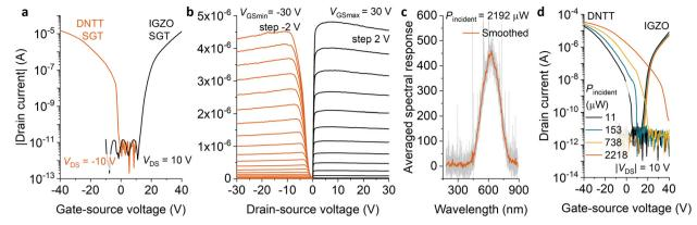
Fig. 2 (a) Transfer and (b) output characteristics for the IGZO and DNTT SGTs having channel widths  $W_{\text{DNTT}}$  = 200  $\mu$ m and  $W_{\text{IGZO}}$  = 90  $\mu$ m. Both transistors operate in enhancement mode, have large on-off current ratio and similar on-state drain currents; (c) measured spectral response of the light source used for photostimulation; (d) transfer characteristics for the IGZO and DNTT SGTs under illumination using the light source in (c) at different intensities.
